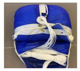
Place the folded suspension lines into the pocket as shown.
