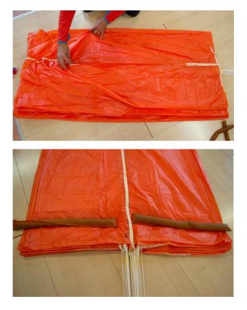
Put a packing weight for fixation on the last panel and than all the panel from the right side can be shifted to the that side.
