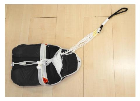
Use the last 20 cm of the suspension lines for the final closing of the inner container with the black rubber.
