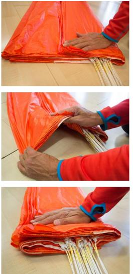
The left third is folded onto the middle and then the right third is folded under the middle. Do the same on top of the canopy.
