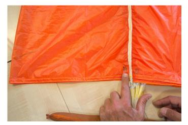
Put all the panets to the right side and fold over each panel from the right side onto left side like turning the pages in a book and pull the top of the opening outward..
