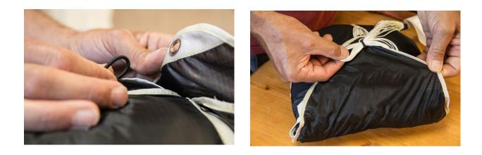
With the rest of the suspension lines you finalize the closing of the inner container by pulling the suspension lines through the black rubber loop. Don't make the closing loop to big.
