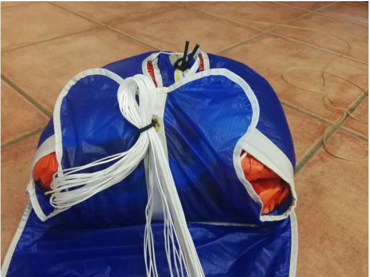
The suspension lines are sorted in bundles, which are fixed by silicon rubbers.
